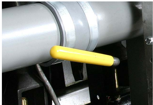
Return filtered oil to the frypot by pulling yellow handle to open oil return valve.
